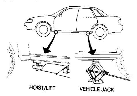
Fig. 1: Locating Hoisting/Lifting Points On Lower Body Seam Courtesy of Subaru of America, Inc.
